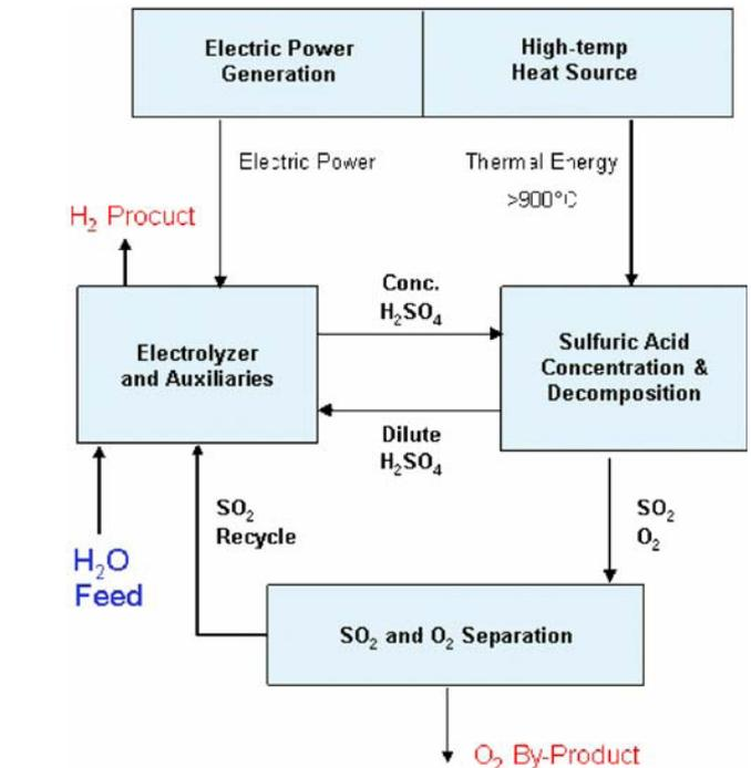
**A simplified flow-sheet of the Westinghouse Sulfur Cycle**
